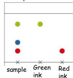
In this example, two known compounds (red and green ink) have been added to the chromatography paper. We can use them to confirm that the unknown sample contains red and green ink because the spots in the sample have travelled the same vertical distance.
